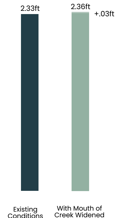
Figure 16: Modeled depth of water on marsh before and after widening the mouth of the creek
